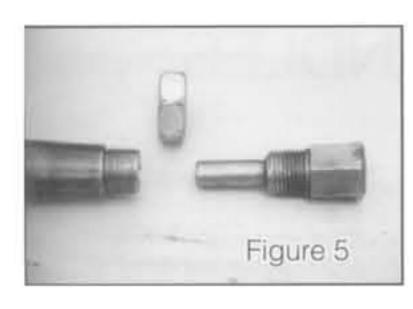
an alternative, you could also use a short 9/16"-18 Grade 5 or Grade 8 bolt and flat washer. However, since this grade bolt is very hard, it is difficult to drill a 25/64" hole through it for the light switch rod.
