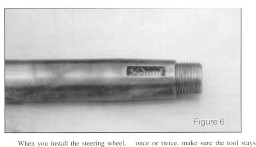
I recommend the use of a new steering wheel nut or use a 5/8"-18 tap to clean up the threads on an old nut so you start with fresh threads.
